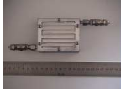
Figure 10 – Condenser shape and overall dimensions.
